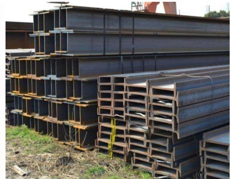
The Parallel Flange Beams come in different shapes depending upon the width & depth of the beam and are generally known as I-beam and H-beam. The H-beam has wider flanges than an I-beam, while the I-beam has tapered edges. Thus the main difference between both H-beams and I-beams is the flange by web ratio. The types beams further vary
